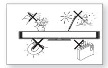
Protect the product from moisture (i.e. vases) , and excess heat (e.g.fireplace) or equipment creating strong magnetic or electric fields Disconnect the power cable from the AC supply if the unit malfunctions. Your product is not intended for industrial use. Use of this product is for personal use only.
